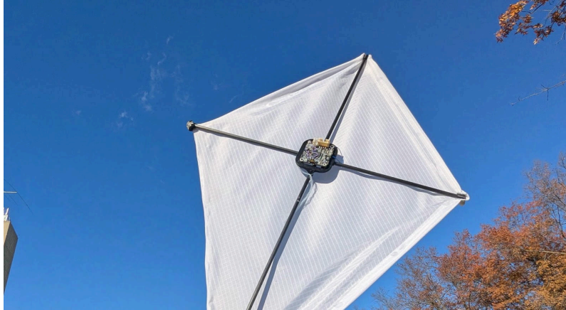
Figure 6: ocularium node mounted on a kite.
